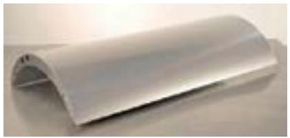
Instead of producing the drum out of massive material the company produces the drums by gluing metal sheets. Material savings are 48%, additional energy savings through reduced weight for the rotating parts.
